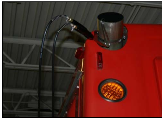
Figure 3.8: Sample lines connected to the tailpipe of the bus
