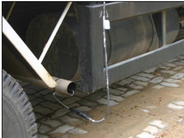
Figure 3.5: Extracting emission from the tail-pipe
